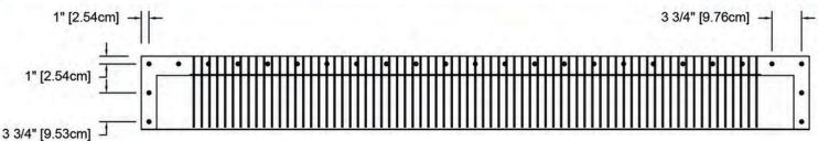
Required screw #10 x 1.5" steel sheet metal screw. With the vent in place secure the flange to the shingle roof using a screw gun or drill. All installation screws are placed at 1" from edge. Number of screws required: 27
