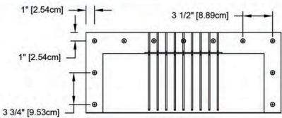
Required screw #10 x 1.5" steel sheet metal screw. With the vent in place secure the flange to the shingle roof using a screw gun or drill. All installation screws are placed at 1" from edge. Number of screws required: 11
