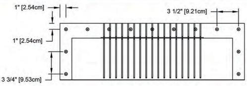
Required screw #10 x 1.5" steel sheet metal screw. With the vent in place secure the flange to the shingle roof using a screw gun or drill. All installation screws are placed at 1" from edge. Number of screws required: 13
