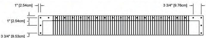
Required screw #10 x 1.5" steel sheet metal screw. With the vent in place secure the flange to the shingle roof using a screw gun or drill. All installation screws are placed at 1" from edge. Number of screws required: 25
