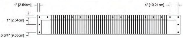
Required screw #10 x 1.5" steel sheet metal screw. With the vent in place secure the flange to the shingle roof using a screw gun or drill. All installation screws are placed at 1" from edge. Number of screws required: 22
