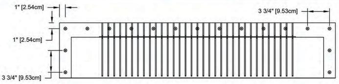
Required screw #10 x 1.5" steel sheet metal screw. With the vent in place secure the flange to the shingle roof using a screw gun or drill. All installation screws are placed at 1" from edge. Number of screws required: 17
