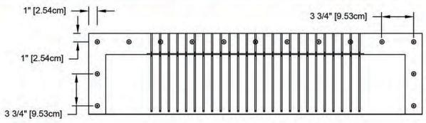
Required screw #10 x 1.5" steel sheet metal screw. With the vent in place secure the flange to the shingle roof using a screw gun or drill. All installation screws are placed at 1" from edge. Number of screws required: 15
