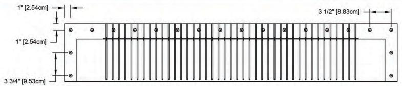
Required screw #10 x 1.5" steel sheet metal screw. With the vent in place secure the flange to the shingle roof using a screw gun or drill. All installation screws are placed at 1" from edge. Number of screws required: 20
